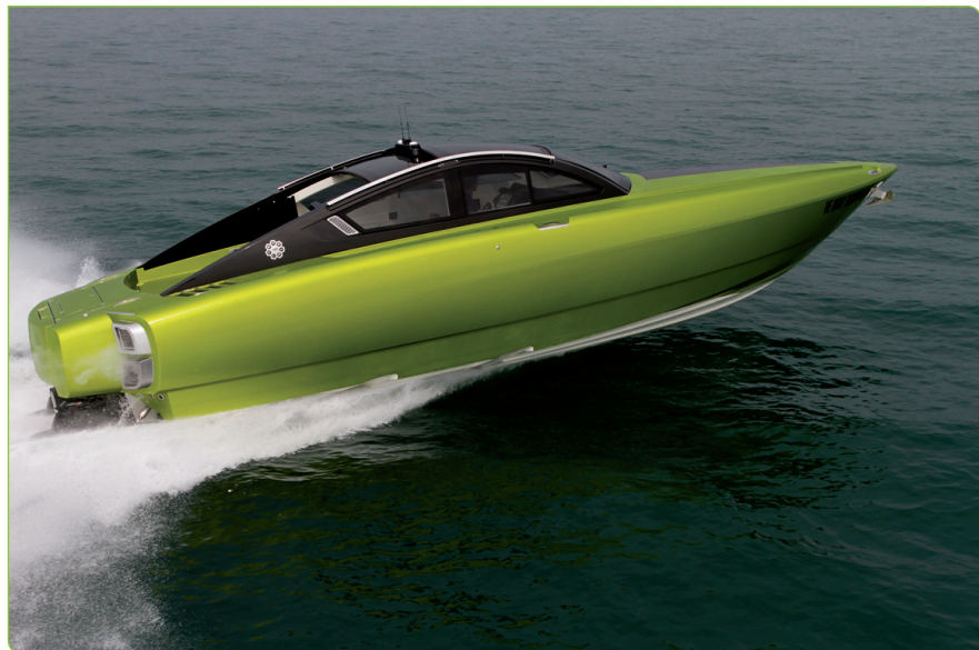
Fig. 1: Due to the use of high-performance composite materials and vacuum infusion, the Revolver 42 speedboat has a dry weight of only 7,500 kg and is capable of speeds of up to 68 knots
