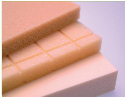
Fig. 2: Corecell™ M-Foam was specified for the sandwich structure as it provides high strength, low density and very low resin absorption to significantly reduce laminate weight
