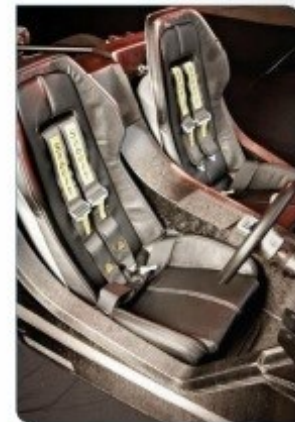
Fig. 3: FR-1 sports car finished cockpit with a carbon fibre composite monocoque chassis
