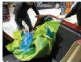
Fig. 2: Demoulding the epoxy/carbon composite monocoque cockpit chassis
