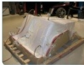
Fig. 1: The carbon fibre epoxy composite monocoque cockpit chassis was moulded out-of-autoclave under vacuum from GMS EP270 epoxy prepreg at only 70°C
