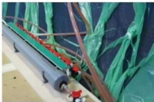
▲ To mould the hull in one shot, several manifolds for the numerous colour coded vacuum lines and resin lines were needed with tags on each resin line
