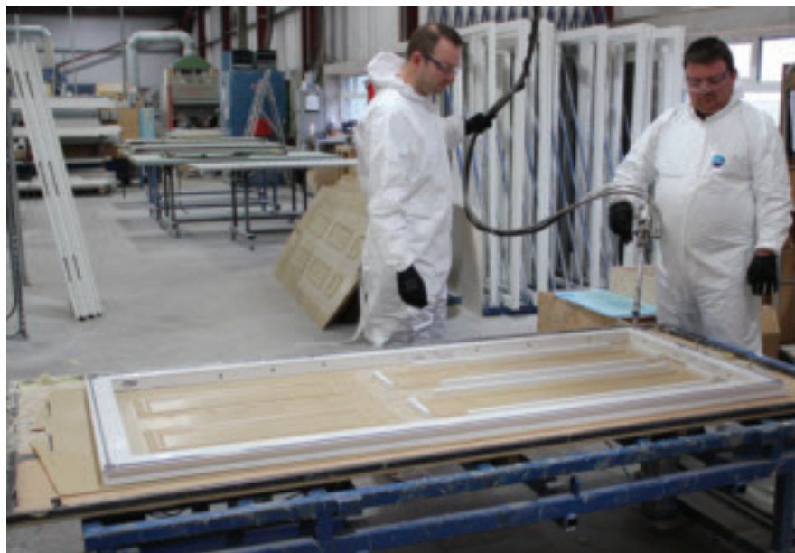
For larger bonding applications, such as fixing door skins to the inner frame, New World applies Crestabond M1-05 from 20 litre pails using an automated 10:1 dispensing machine.
