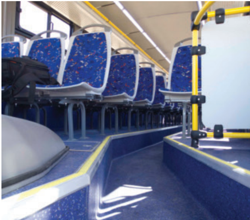
The aisle GRP flooring sections are bonded into the bus chassis structure using Crestabond M1-20, which is also used to bond metal fittings on GRP ceiling and side panels.
