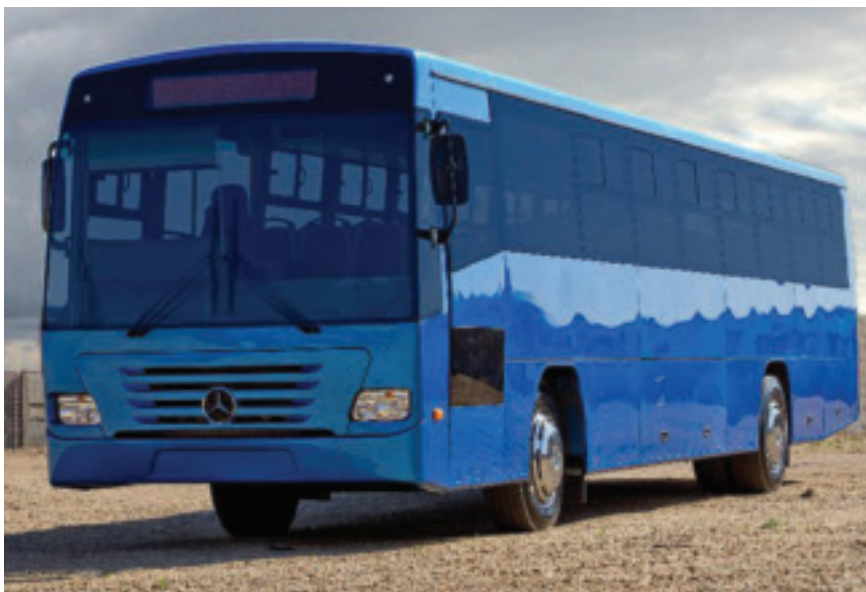
Busmark 2000 manufactures GRP front and rear domes and exterior cladding for Mercedes Benz buses, which are now bonded in preference to using mechanical fixtures.
